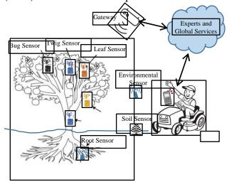
FIGURE 5: An IoT based Farm Area Network (FAN)
