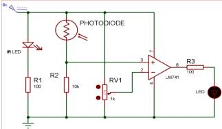
FIG.1 Circuit Diagram of IR Sensor
