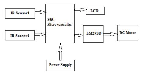
Fig. 3 Block Diagram of Railway Gate System
