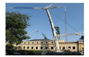
A telescopic crane has a boom that consists of a number of tubes fitted one inside the other. A hydraulic or other powered mechanism extends or retracts the tubes to increase or decrease the total length of the boom. These types of booms are often used for short term construction projects, rescue jobs, lifting boats in and out of the water, etc. The relative compactness of telescopic booms makes them adaptable for many mobile applications.
