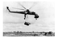
Aerial crane or 'Sky cranes' usually are helicopters designed to lift large loads. Helicopters are able to travel to and lift in areas that are difficult to reach by conventional cranes. Helicopter cranes are most commonly used to lift units/loads onto shopping centers and high rises. They can lift anything within their lifting capacity, (cars, boats, swimming pools, etc.).
