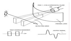
Figure 3 IR motion sensor
