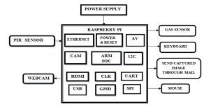
Figure-1 Proposed Block Diagram
