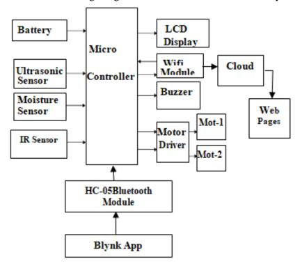
Figure 1: Block diagram of Garbage Collection and Monitoring Robot Using Wireless Communication
