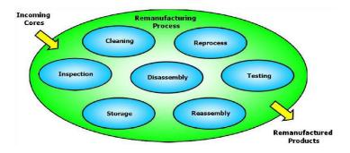
The step 'reprocess' stands for machining operations, toner loading, or whatever else is needed to make the product usable again. This step is determined by the type of commodity being remanufactured.
