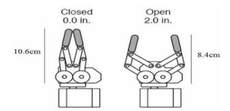
Figure 4 Robotic Arm Architecture
