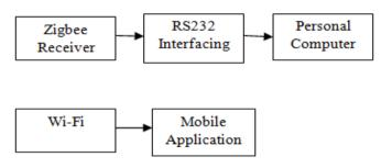
Figure 6 Receiver Section
