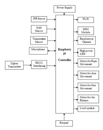
Figure 3 Block diagram of Transmitter Section
