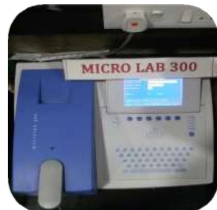
SEMI-AUTOMATED CLINICAL CHEMISTRY ANALYZER
