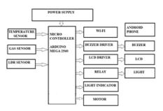
Figure 1: Block Diagram
