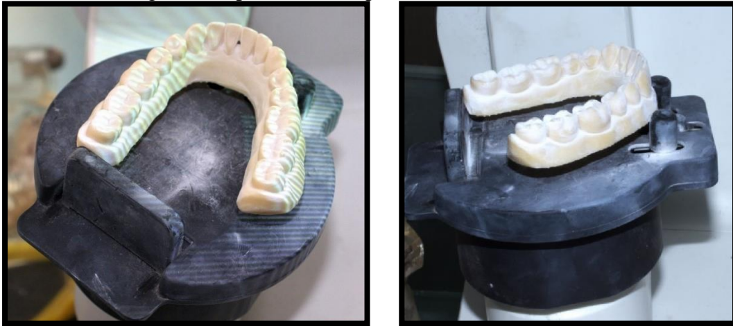
Fig. 19 (a), (b) : 3D printed model being scanned using the desktop scanner
