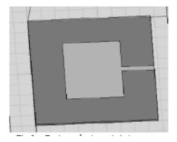
Fig 2: Rectangular type-1 Antenna
