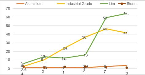
According to the above results, while adding 3g of the stone alum in, it 300ml of sample gives the better results than others. So, it is chosen as the optimum dosage. The dosage is selected as 10g/l to treat the water.
