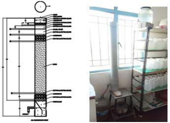
Fig.5 Layout of filter media
