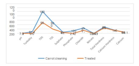
Fig.10 Comparison between waste water and treated water
