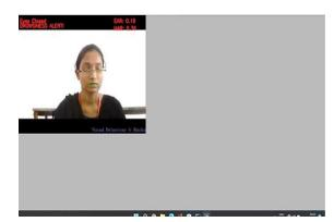
The position of mouth is calculated by using MOR Mouth opening ratio is a parameter to detect yawning during drowsiness. Similarly, if mouth starts to yawn, then also will get drowsiness alert message and rings an alarm and keep on counting the number of yawns.
