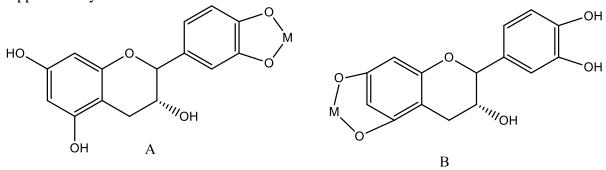
Figure 2: Proposed structure of L-Catechin-Metal complexes
