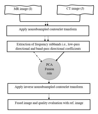
Fig. 2: PCA-based NSCT image fusion system.
