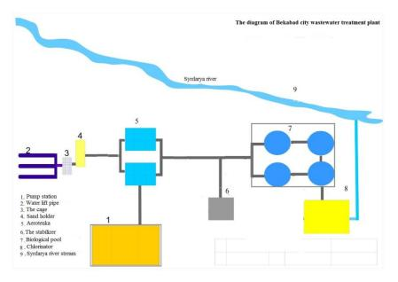
Figure 2. Drawing of the Bekabad city wastewater treatment plant
