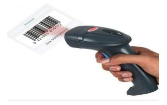
Fig. 3.1 Barcode Scanner
