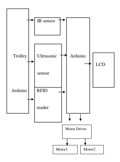
Fig. 5.1 System architecture
