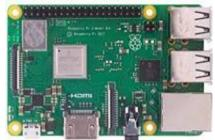
Figure 2:Raspberry Pi 3 Model B+
