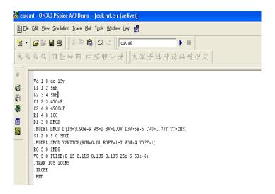
Figure 3.2: Pspice program for Cuk converter circuit.
