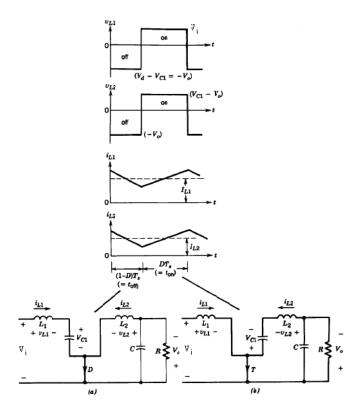
Figure 2.3: Cuk converter waveforms (a) switch off (b) switch on.
