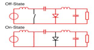
Figure 2.2: two operating states of Cuk converter.
