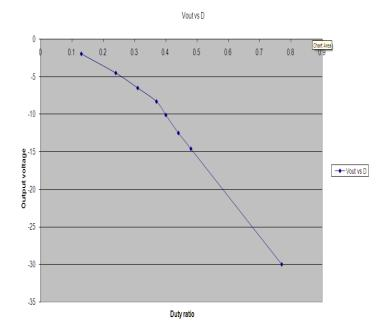
Figure 4.6: Output voltage Vs Duty ratio at constant input voltage & variable loads Vi = 15volts Ro = 250 or 100 ohms.
