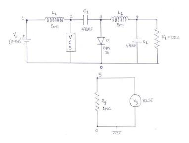
Figure 3.1: Cuk Converter simulation circuit diagram.
