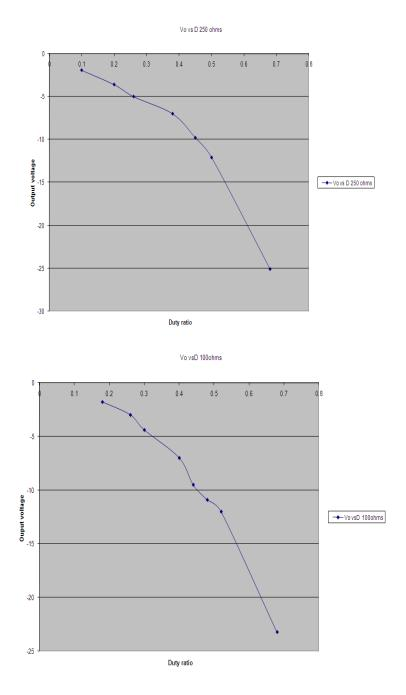
Figure 4.8: Output voltage Vs Duty ratio at variable input voltage & constant loads.
