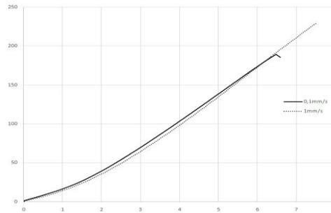
Figure 3: Experimental stress-strain curves for BFRP specimens
