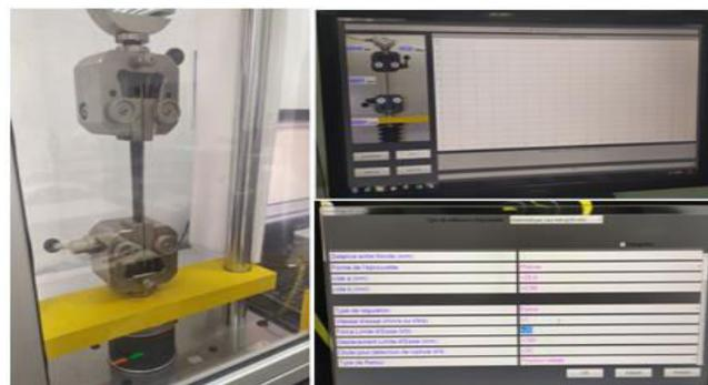
Figure 2: Setup used for traction test
