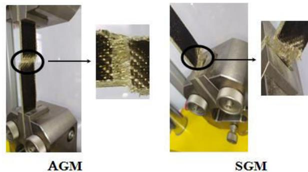
Figure 6: Bulk images of BFRP composite with different failure
