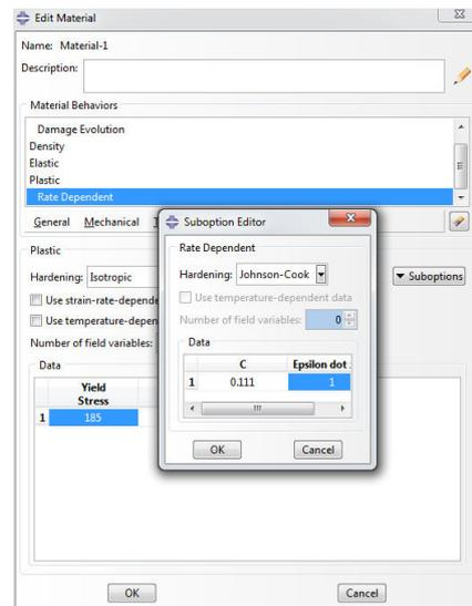
FIGURE 7: SIMULATION OF STRAIN 1 MM/S DYNAMYC (JHONSON COOK)
