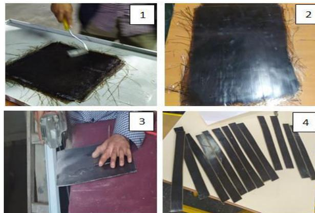
Figure 1: Fabrication process of specimens
