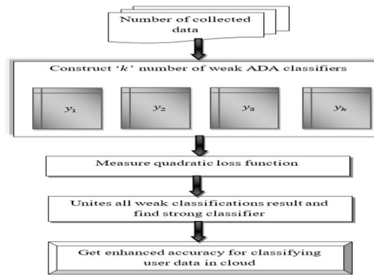
**Figure 2 Block Diagram of Adaptive Discriminant Quadratic Boosting Ensemble Classifier**
