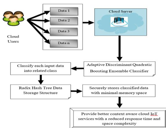
**Figure 1 Architecture Diagram of ADQBC-RHCDS Model for Context Aware Cloud IoT Services**
