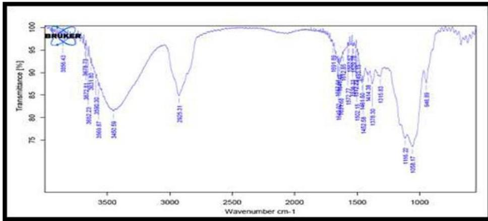
fig.3 (a): IR Spectrum of 1[2[(4chlorophenyl)methoxy]2(2,4dichlorophenyl)ethyl]imidazole ;nitric acid
