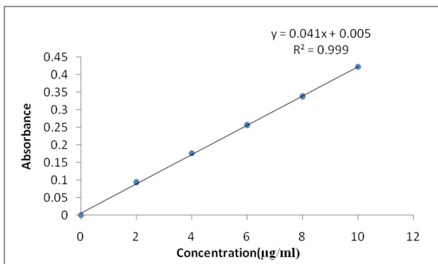
**fig.2:-** Calibration curve of Econazole nitrate in methanol
