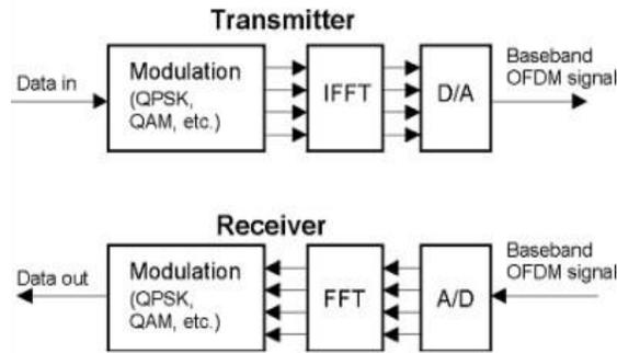
**Fig1. Basic FFT, OFDM Transmitter and Receiver. Design of OFDM\_Tx:**
