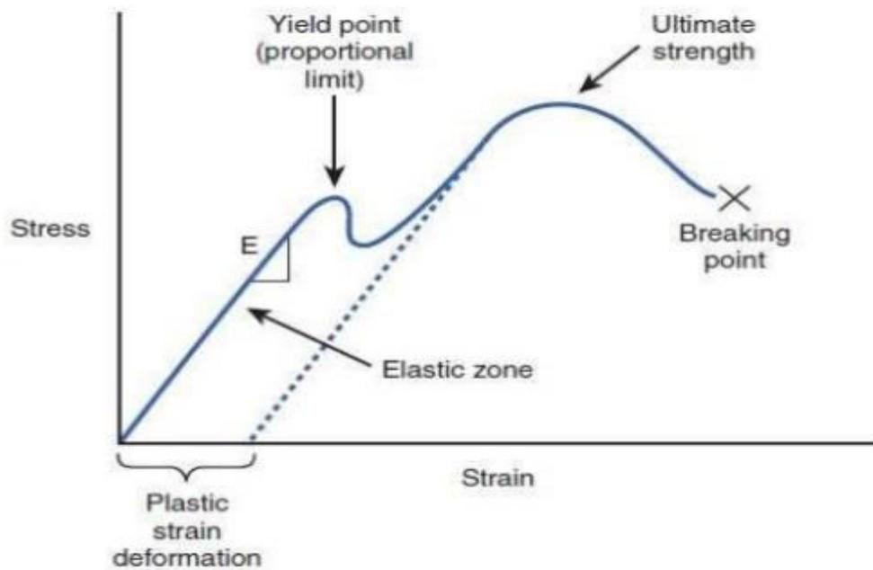
**Figure (7):** shows stress strain curve of the material of the interlocking nail (5)
