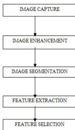
Fig 1: Flow Process in MIP
