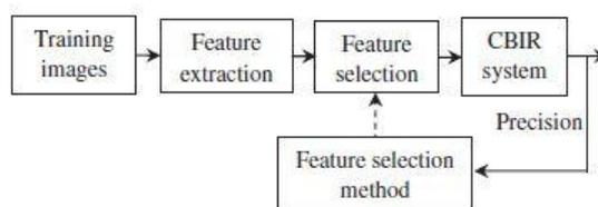
Fig 2: Block Diagram of a CBIR system
