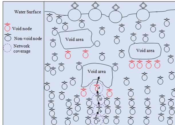
Fig 1. Illustration of Communication Void in UWSN
