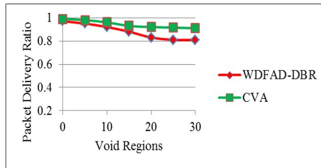
Fig. 5 Packet Delivery Ratio of Various Void Regions at 500 Nodes
