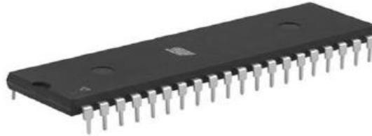
Fig. 7 Microcontroller AT89C51
