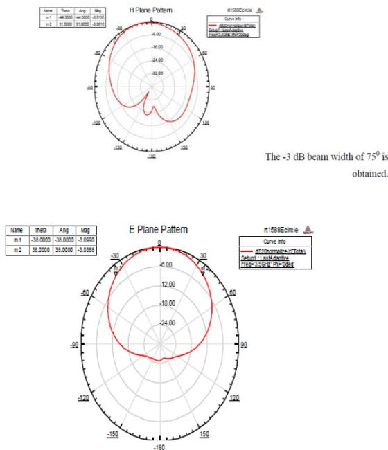
Figure7 E plane pattern of CMPA with edge feed.
