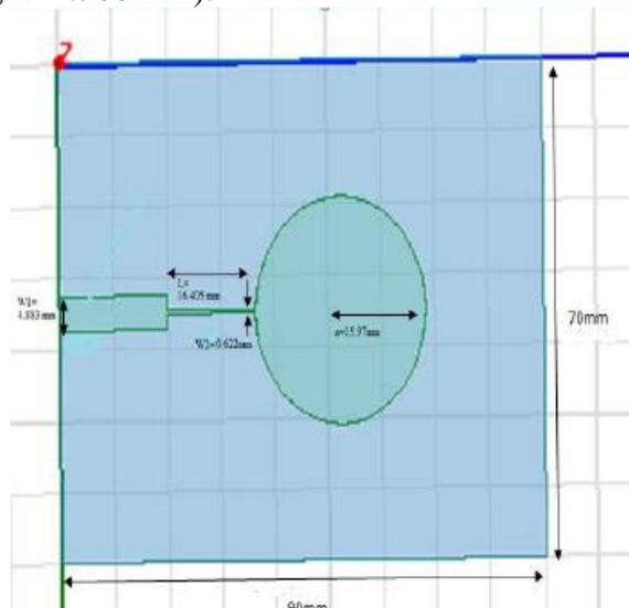
Figure4 Edge feeding of CMPA with all dimensions
