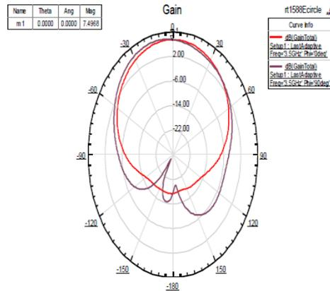
Figure.8 Gain pattern of CMPA with edge feed.
