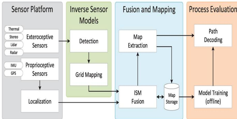
Fig-1 Flow diagram of the synergistic fusion for concurrent environment mapping and moving object detection.
