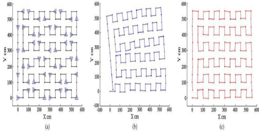
Fig. 3. Reenactment for graph-based ideal estimation. (a) reproduction from claiming genuine robot trajectory. (b) robot trajectory estimate utilizing a odometer. (c) robot trajectory arrangement then afterward MLE.
