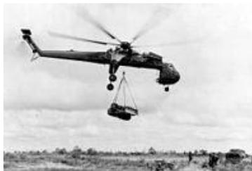
Aerial crane or 'Sky cranes' usually are helicopters designed to lift large loads. Helicopters are able to travel to and lift in areas that are difficult to reach by conventional cranes. Helicopter cranes are most commonly used to lift units/loads onto shopping centers and high rises. They can lift anything within their lifting capacity, (cars, boats, swimming pools, etc.).
