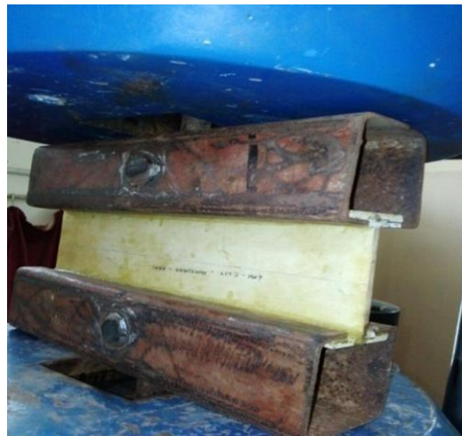
Tensile Testing of 3rd I-Beam specimen with 4mm cleat
