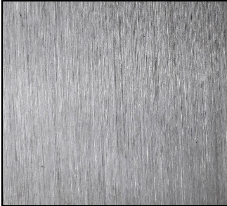
Figure 1: SEM evaluation of Group I samples illustrating several finer and dense closely packed striations
