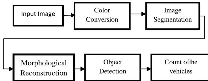
Fig.1. Block diagram of Vehicles Detection from Satellite Images using Digital Image Processing
