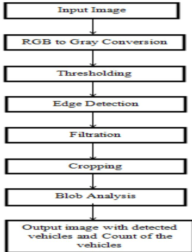
Fig.2. Flowchart representation of vehicles detection from satellite images using digital image processing
