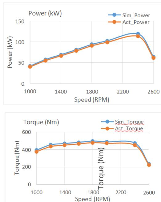
Figure.11. Compare MPFI system from GT power analysis
