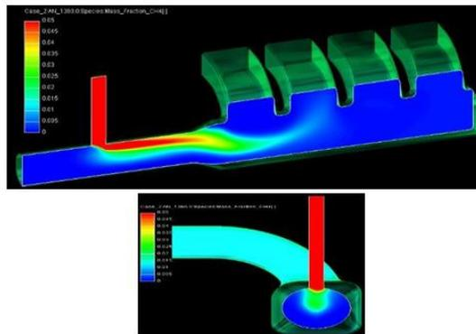
Figure.3. The simulation of 3D CFD for the configuration of SPFI
