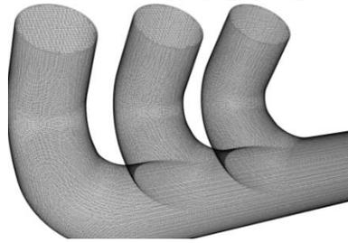
Figure.2. Mesh Geometry of Intake Manifold
