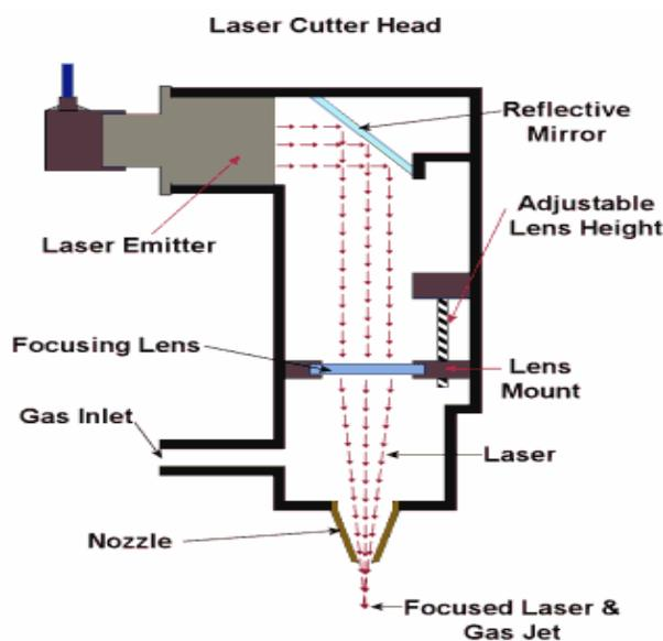
Figure .5. Laser cutting technology
