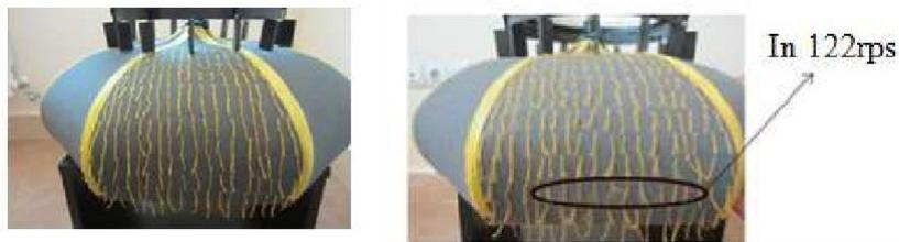
a) Tufts flow visualization technique b) Flow separation point
