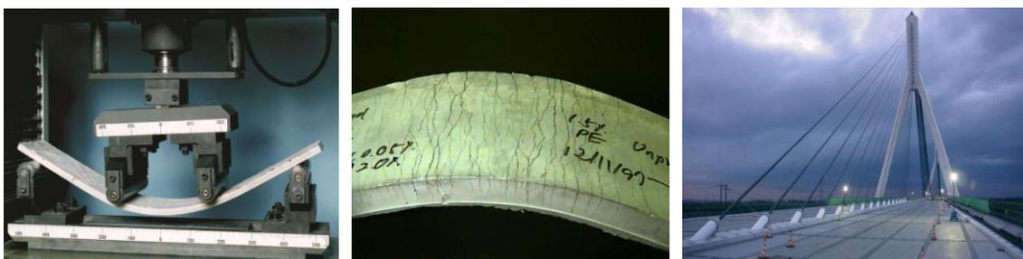
Figure 5: (a), 4 Point Flexural test on a concrete slab, (b) Concrete slab after flexural test (cracks
