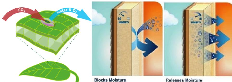
Figure 2: (a) Carbon dioxide enters, while water and oxygen exit, through a leaf's stomata - graphical image, (b) MemBrain blocks moisture – during winter, (c) MemBrain releases moisture - during summer
