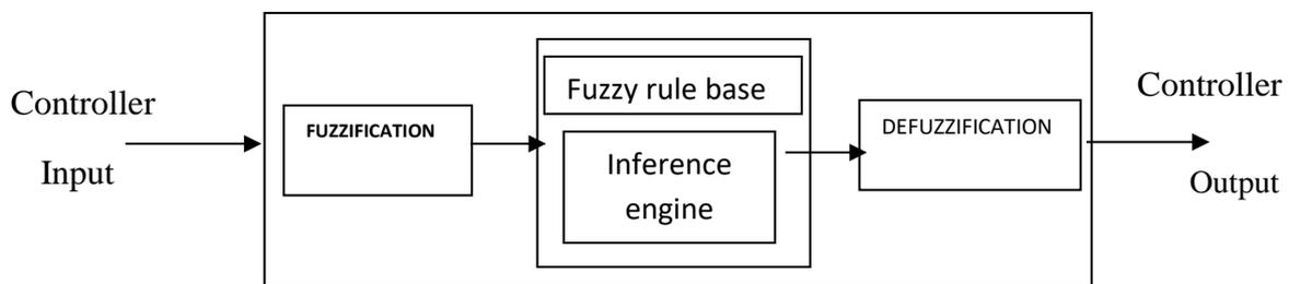
**Fig. 2: Block diagram of fuzzy control system**
