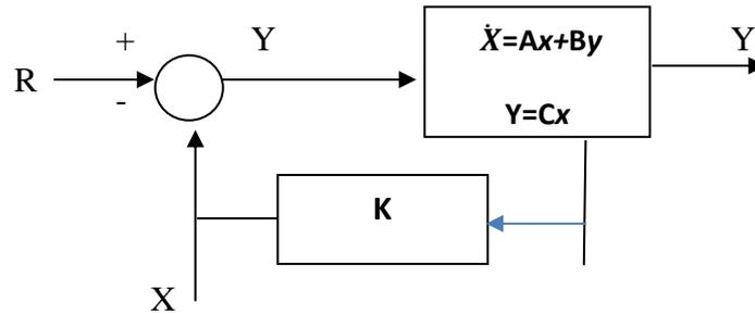
**Fig.3. Optimum feedback controller of LQR**
