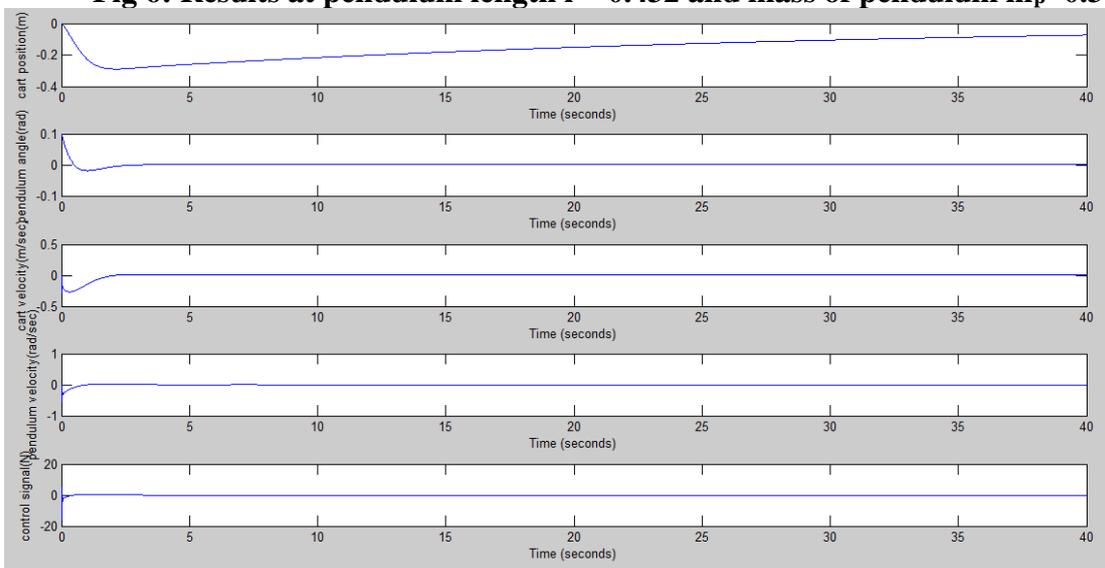
**Fig 7: Result of Inverted pendulum at pendulum length  $l=0.36$  mass of pendulum  $m_p=0.72$**
