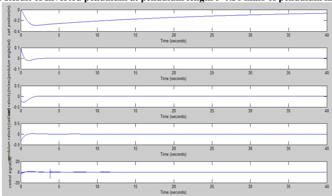
**Fig 8: Results at pendulum length  $l=0.432$  and mass of pendulum  $m_p=0.72$**
