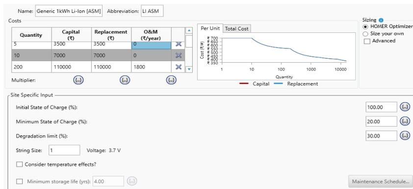
Figure.6. Battery cost optimiser in HOMER
