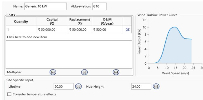
Figure.5. wind turbine cost optimiser and power curve in HOMER
