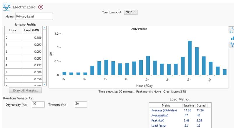
Figure.7. Daily electric load profile optimiser
