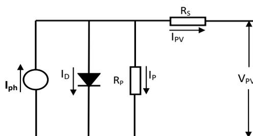
Figure. 3. PV Cell equivalent circuit
