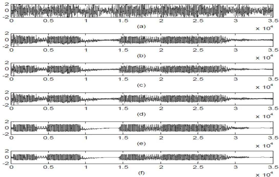
Fig.3: Helicopter Noise Removal Filtering Results for Sample – I (a) Contaminated Speech Signal, (b) Using LMS Algorithm recovered signal, (c) Using DVLMS Algorithm (d) Using EVLMS Algorithm (e) Using TVLMS (f) Using SVLMS Algorithms.
