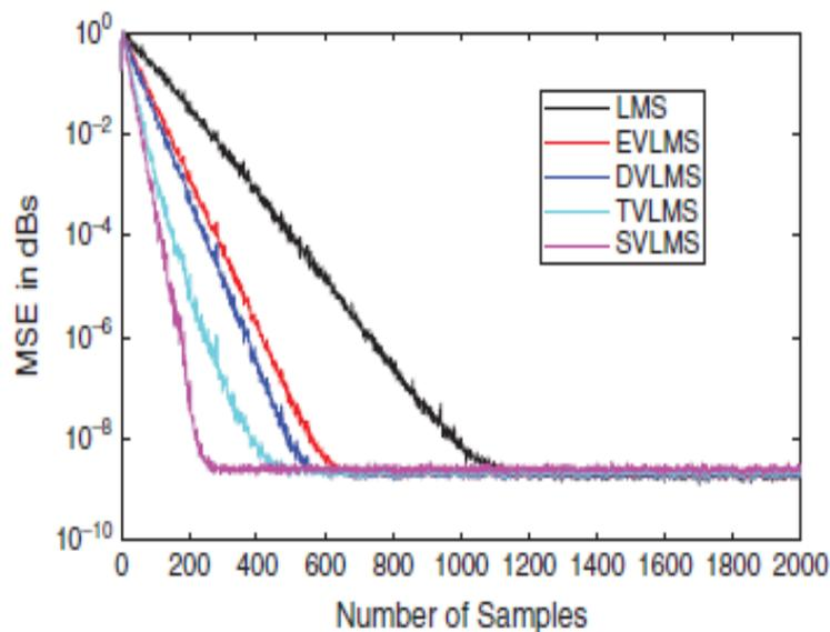
Fig. 2: Convergence characteristics of LMS and variable step size algorithms
