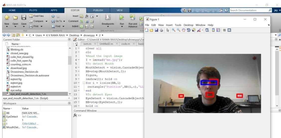
Fig 2: When the driver's image is uploaded, the inbuilt software recognizes his image and divides his image into respective parts like nose mouth and eyes.
