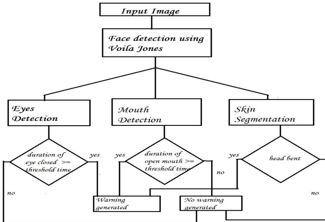
Fig 1: Flow Diagram for working of the detection system
