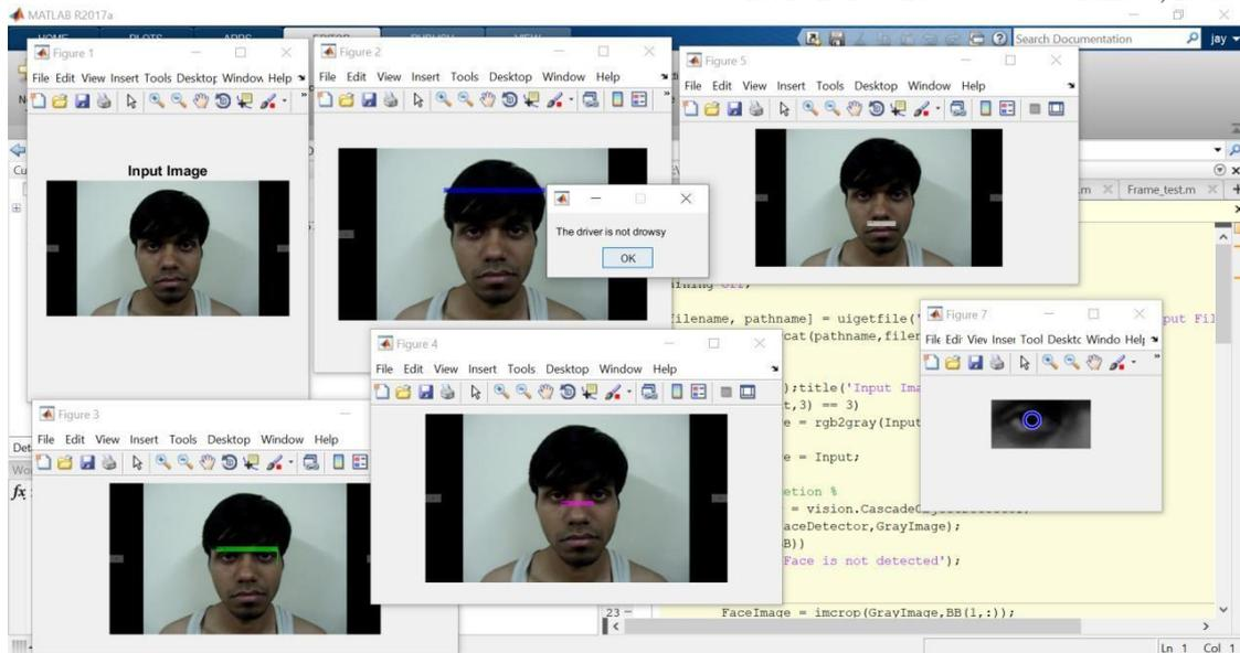
Fig 5: If the person image which is uploaded is detected that the person is not drowsy then the output is an alert box which displays that the person is not drowsy
