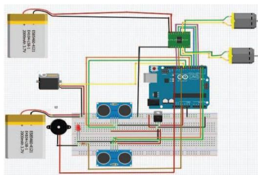
Fig.2. Implementation of prototype using Arduino
