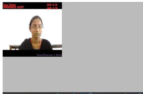
The position of the mouth is calculated by using MOR. Mouth opening ratio is a parameter to detect yawning during drowsiness. Similarly, if the mouth starts to yawn, it will also get a drowsiness alert message and ring an alarm and keep on counting the number of yawns.
