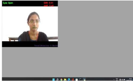
It keeps on counting the score by observing the eye aspect ratio. If the obtained values for a person's eyes are compared with the threshold values. As the person's eyes are closed for a few seconds i.e., reached the threshold values, it shows a drowsiness alerting message and alerts him by ringing an alarm.
