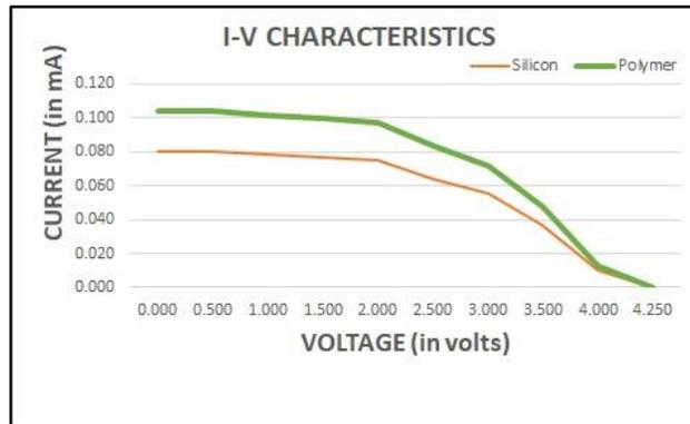
Fig 13. Current Vs Voltage Comparison Graph
