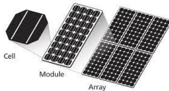
Fig 2. A Solar Cell, Solar Panel & Solar Array
