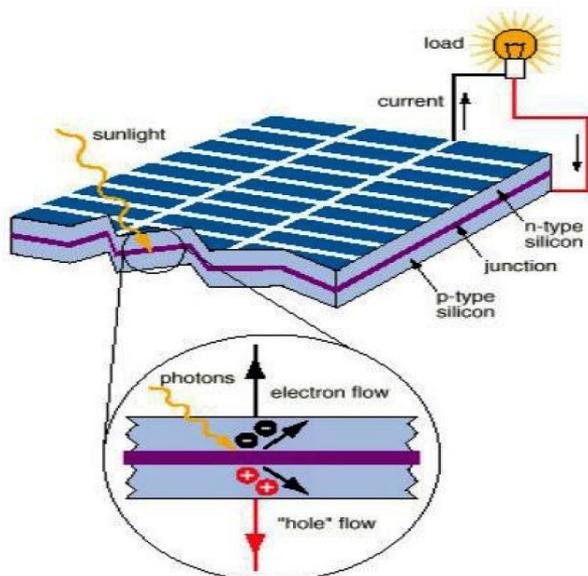
Fig 5. Si-Solar Panel Functioning Principle
