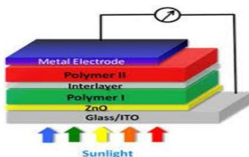
Fig 6. Structure of a Plastic Solar Cell
