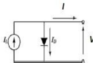
Fig 11. A single diode equivalent circuit for an ideal solar cell
