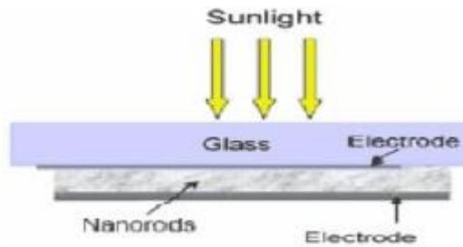
Fig 9. Schematic of a Plastic Solar Cell
