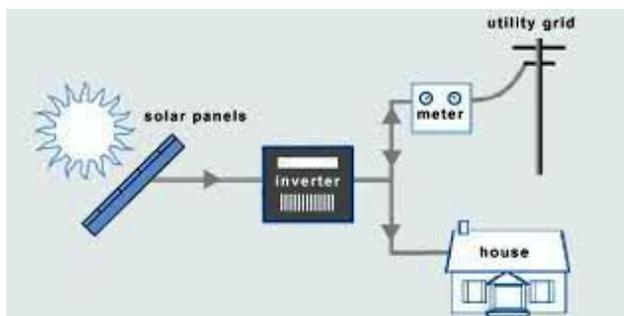
Fig 4. Grid-Connected PV System
