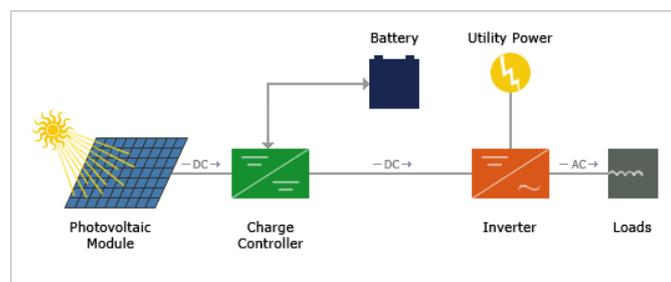
Fig 3. A Stand-Alone PV Module
