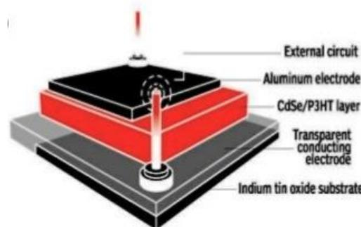
Fig 10. Operation of a Plastic Solar Cell
