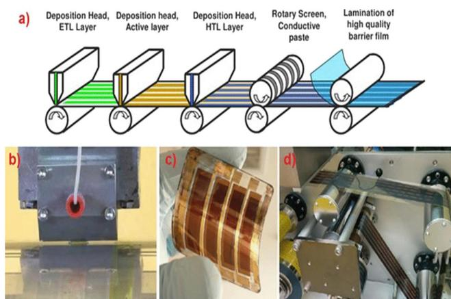
Fig 8. Screen Printing of Plastic Solar Cells
