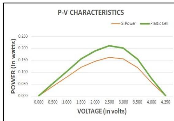
Fig 14. Power Vs Voltage Comparison Graph
