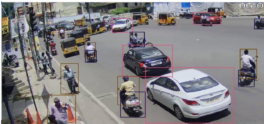
Fig.3 Extraction of motorbikes from surveillance video using YoloV3 Algorithm.
