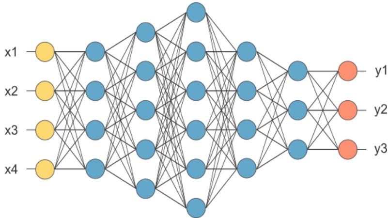
Fig.2 Fully Connected Layer
