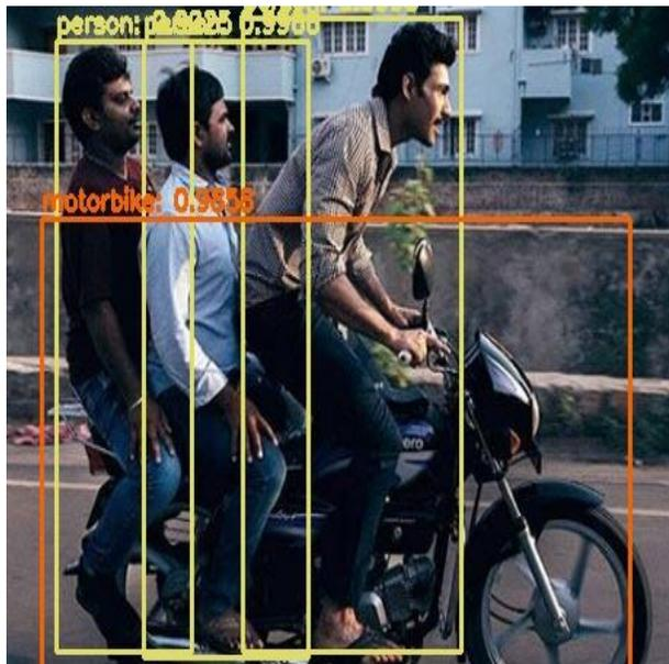
Fig. 5 Detection of triple riding using CNN-YoloV3
