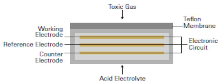
**Figure 1. Working model of Electro chemical sensors**
