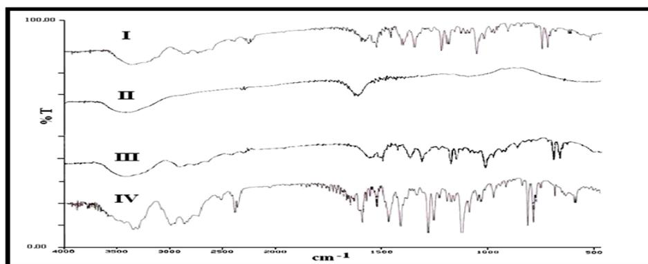
**Figure 6 FT-IR spectra of pure Propranolol hydrochloride (I), HPMC (II), ethyl cellulose (III), and Optimized formulation F7**
