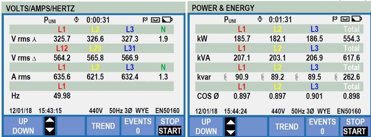
Fig: 4 Power Factor, Active Power, reactive power reading without SVC installed.
