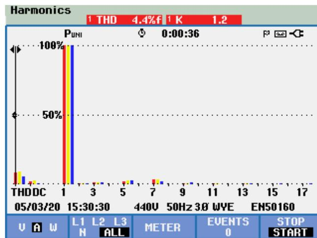
Fig: 9 Harmonics reading with SVC on Dt. 05.03.2020
