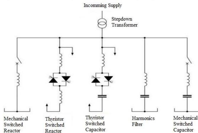
Fig: 3 Static VAR Compensator (SVC)
