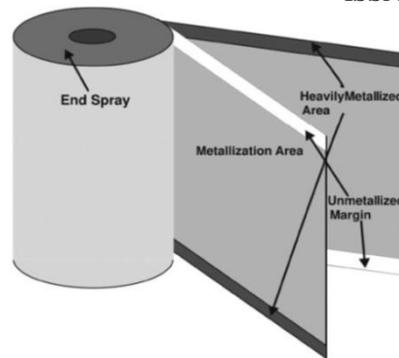
Fig: 1 construction of Metallized film capacitor (MPP)
