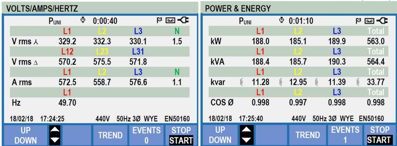
Fig: 6 Power Factor, Active Power, reactive power reading with SVC on Dt. 18.2.2018
