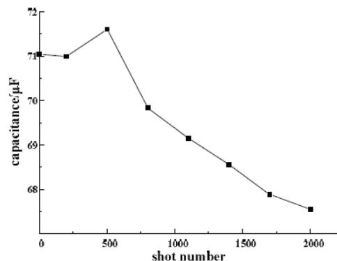
Fig: 2 Effects of no. of faults on Metallized film capacitor
