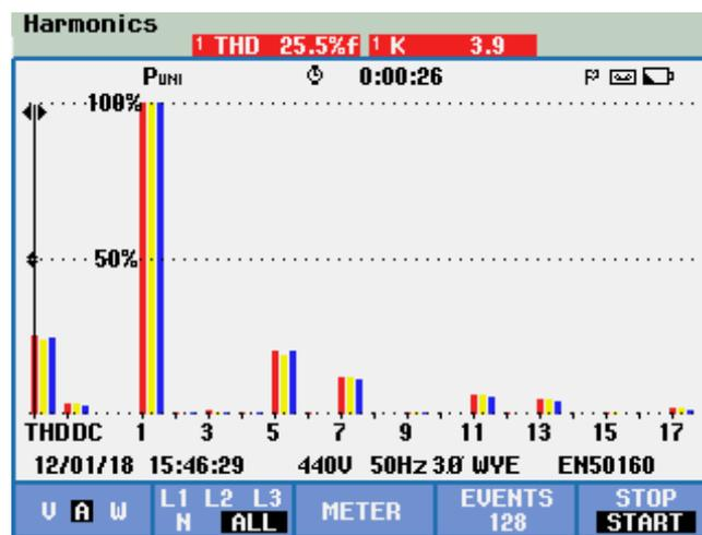
Fig: 5 Harmonics reading without SVC installed
