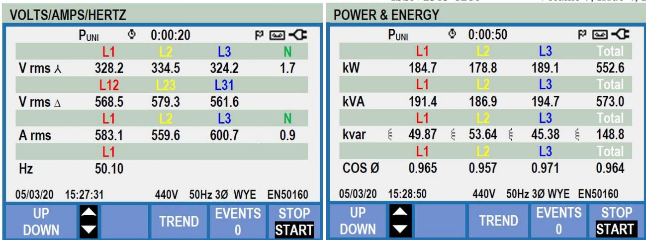
Fig: 8 Power Factor, Active Power, reactive power reading with SVC on Dt. 05.03.2020
