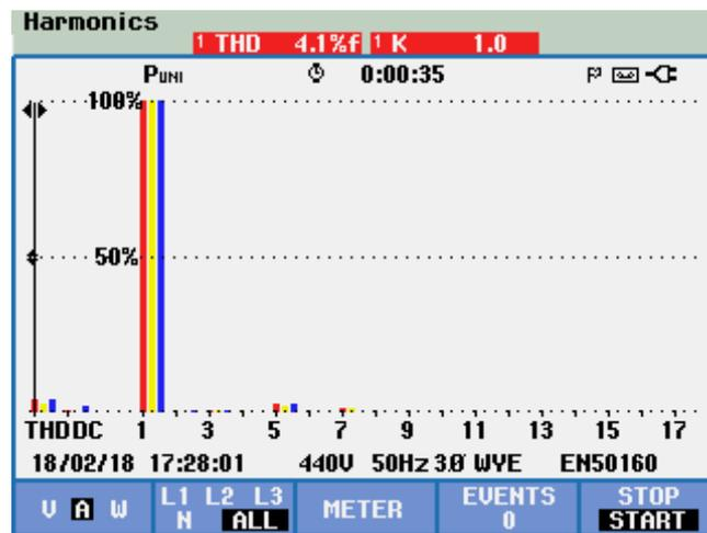
Fig. 7 Harmonics reading with SVC on Dt. 18.2.2018
