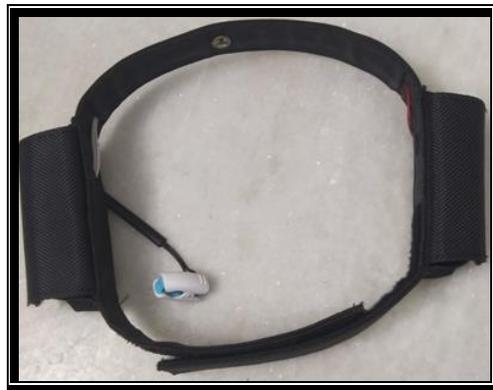
Fig 1.2 Brain wave detecting headset
