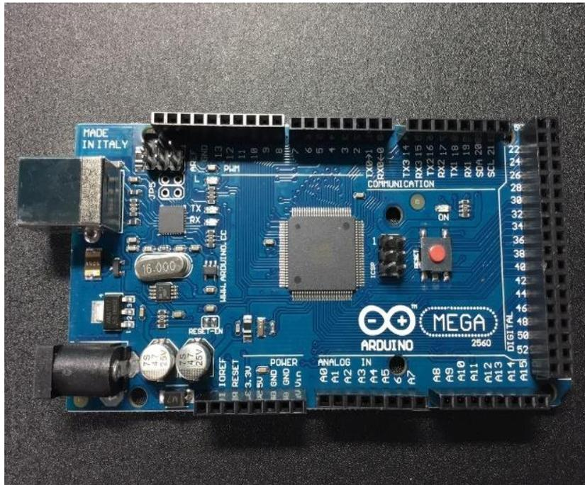
**Fig 2:Arduino Mega 2560**
