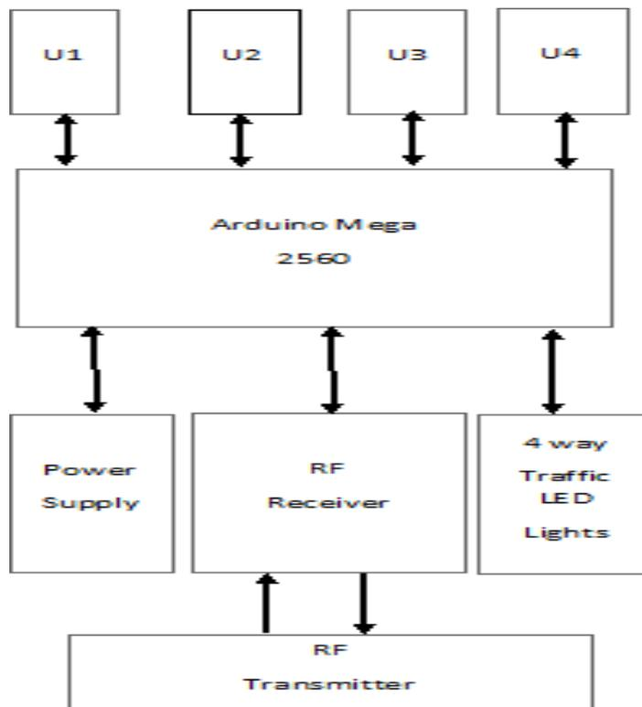
**Fig 3: Four Way Traffic LED using Arduino**
