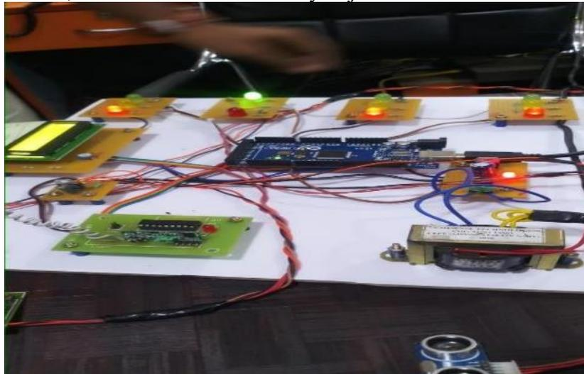
Fig 1: Operation model of Density Based Traffic signal using Arduino.
